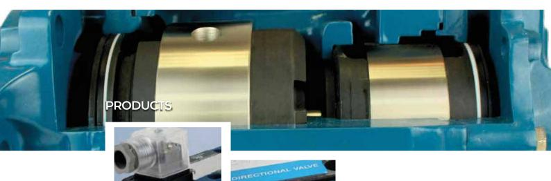
TDZ Hydraulics introduces the most complete line of fixed displacement vane pumps, both for mobile and industrial applications. Hydraulically balanced, our pumps offer low noise level and high volumetric efficiency.
